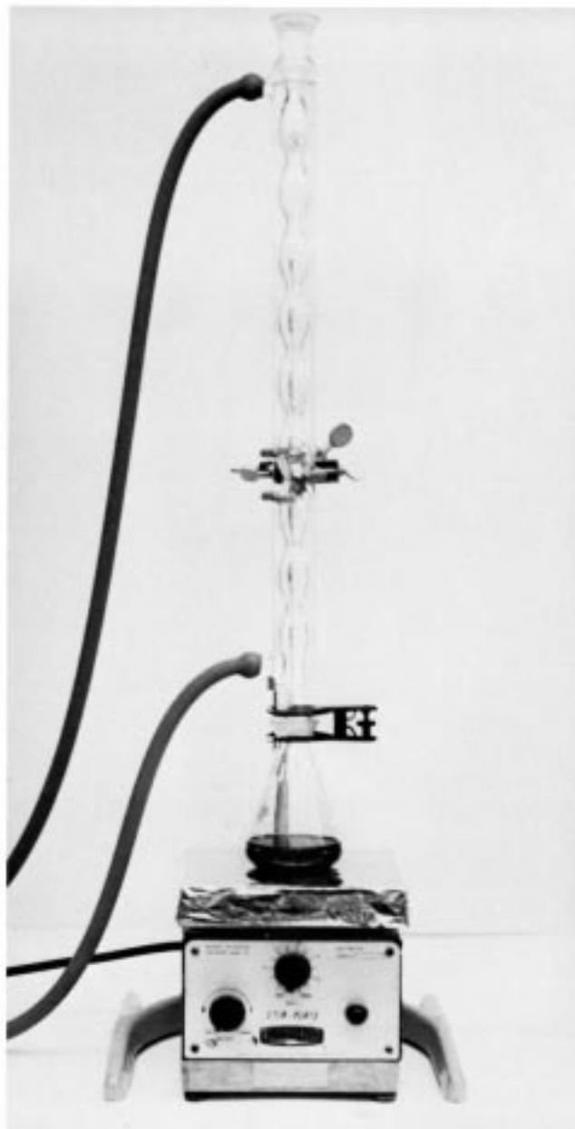
FIG. 1 Dispersing Apparatus
